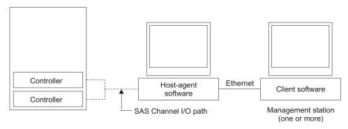
Note: The client software is installed on one or more management systems, or on the host computer.
